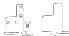
Corner bearing 6-25337-00-L-1 Cover 9-32513-00-L- Screw 9-38217-00-R-1
