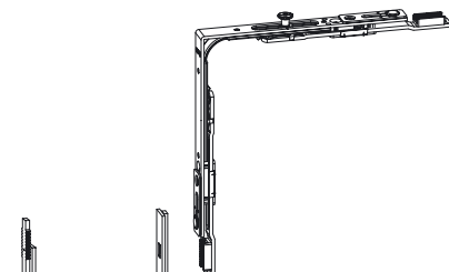
Corner transmission Locking plate acc. to profile
